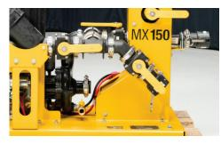
JOBSITE FLEXIBILITY. Hook up the hose from the mix system to the drill on the back or side of the machine.
