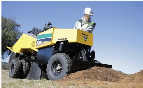
**OPTIONAL HYDRAULIC PUSH BLADE.** The optional hydraulic push blade on the SC382 simplifies jobsite cleanup by helping maneuver processed material.
