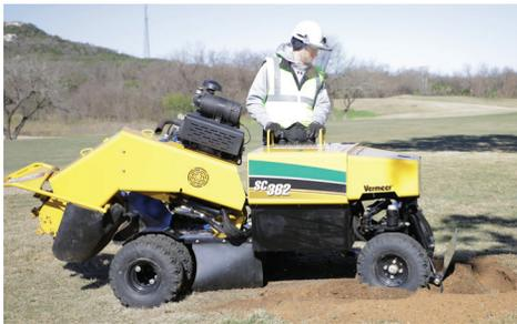
**STANDARD FOUR WHEEL DRIVE.** Four-wheel drive comes standard on the SC382. It offers traction and maneuverability in difficult transport conditions.
