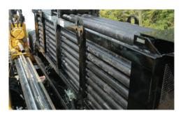
MORE FEET ONBOARD. Install more feet and save time with an impressive 500' (152.4 m) of drill rod on-board.
