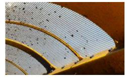
STAINLESS STEEL SCREEN OPTION. Stainless steel screens offer increased durability and reduce the amount of screen binding when working wet or corrosive materials.
