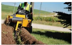
**DEPTH-CONTROL.** Elimination of the tail wheel on the track unit provides trenching depth-control in uneven ground conditions and convenience to move through tight spaces.
