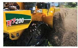
HIGH-TORQUE DIGGING. The RTX200 is equipped with a 20.5 hp (15 kW) Kohler engine for optimal power on your jobsite.
