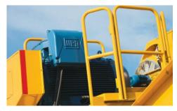
**ELECTRIC MOTORS.** Equipped with a 500 hp (373 kW) WEG totally enclosed, fan-cooled electric motor to power the mill. A separate 50 hp (37.3 kW) electric motor powers the pump for the hydraulic circuits, while a 2 hp (1.5 kW) electric motor powers the fan to cool the hydraulic system.
