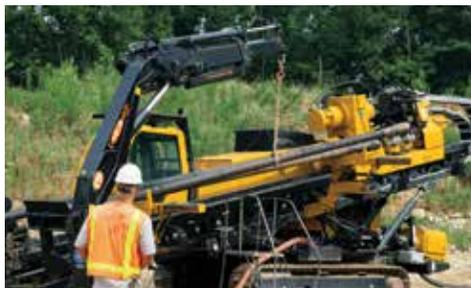
**KNUCKLEBOOM CRANE.** Optional knuckleboom crane mounted on either side of the base anchor easily maneuvers heavy tooling, reducing need for support equipment.
