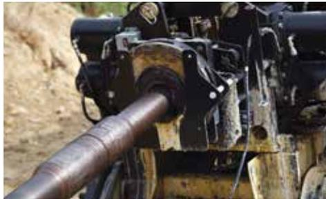
**WISE.** The sliding vise moves 35.4" (89.9 cm) to help operators position the vise for maximum efficiency when reaming or pulling product.
