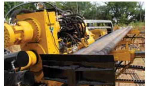
**ROD LOADER.** A single row, sliding arm rod loader allows for the staging of five rods at one time, increasing boring efficiency by minimizing rod loading time.
