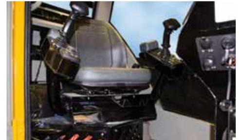
**COMMON CONTROLS.** The D220x300 shares common controls with other drills in the Navigator lineup, decreasing operator training time and allowing for faster startups.
