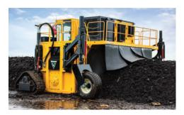
**CLEAN JOBSITE.** Operator controlled rear curtain helps maintain a clean jobsite while windrow shift is minimized by the curtain keeping material in place.
