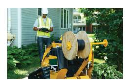
**OPTIONAL REEL CARRIER.** Add an optional reel carrier for increased productivity and efficiency.
