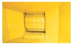
TWIN HORIZONTAL FEED ROLLERS. The lower feed roller is offset from the upper feed roller to ensure that material at maximum capacity is easily fed to the chipper.
