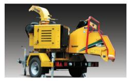
OPTIONAL 180° SLEW RING. Allows the chipper infeed chute to be rotated to face where the material is located for ease of feeding and helps increase safety when working along the roadside by keeping the operator away from road traffic.
