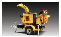
**COMPACT SIZE.** When equipped with all machine options and a full fuel tank, the BC230xL still weighs less than 2000 kg (4409.3 lb). The relatively low weight reduces load on towing vehicle and the 1,9 m (6.2') wide trailer frame provides stable towing performance and good visibility when reversing.
