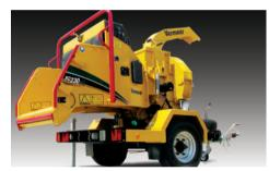
HIGH GROUND CLEARANCE. 36 cm (14.2") under the chassis and 26 cm (10.2") under the axle allows the chipper to be used off-road without risk of ground debris becoming caught and causing damage or problems with towing.
