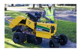
TWO-SPEED GROUND DRIVE. The operator may choose to operate in a high-range or low-range ground speed setting of 0-133 fpm (0-40.5 m/min) to quickly move the machine or choose a slower speed when near the stump by utilizing a low-range setting of 0-66 fpm (0-20.1 m/min).
