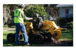
POWERFUL STUMP REMOVAL. A 35 hp (26.1 kW) Vanguard engine offers low vibration, low emissions, smooth easy starting, extended starter life and an instant return to maximum power. Also offers a limited three-year warranty from Vanguard.
