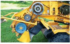
**CONVENIENT BELT SERVICING.** Belts on the SC362 are serviceable from one side of the machine with cutter drive belts being adjustable with movable idlers. Additionally, each belt set may be adjusted independently, without affecting adjustment of other belts.
