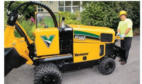
**AUXILIARY CONTROL STATION.** In narrow jobsite conditions that restrict use of the main control station, the operator can control ground drive and steering functions from this folding station mounted at the front end of the machine.
