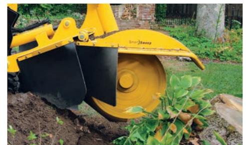
**SMOOTH OPERATION.** The exclusive SmartSweep™ control system monitors engine load and provides continuous feedback, resulting in a smooth and consistent cutter wheel sweep rate.
