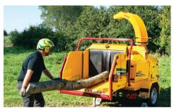
**OPERATOR SAFETY.** Mounted over the feed table, the four-position upper feed control bar enables the operator to stop the feed rollers and select forward or reverse. The patented bottom feed stop bar is strategically located to make it possible for an operator's leg to strike the bar and shut off the feed mechanism either intentionally or automatically in an emergency situation.
