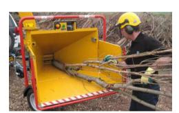
HIGH-CAPACITY INFEED. The BC160xL has a 16 cm x 20 cm (6.3" x 7.9") infeed opening to help boost productivity by reducing the need to trim material before feeding into the chipper.
