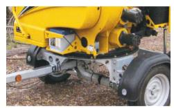
360° ROTATING TURNTABLE. Allows the chipper infeed to be rotated to face where the material is located for ease of feeding and greatly increases safety when working along the roadside by keeping the operator away from road traffic.
