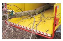
BOTTOM/SIDE FEED STOP BARS. The bottom/side feed stop bar system is strategically located to make it possible for an operator to strike the bar and stop the feed, either intentionally or automatically in an emergency situation.
