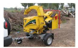
**COMPACT DESIGN.** With a towing weight of just 750 kg (1653.5 lb) and a 276.1 cm (108.7") transport length, the BC160xL is compact for small jobsites, yet has an ability to take on large material. The discharge chute folds easily from a working height of 240 cm (94.5") to 193 cm (76") for transport and storage.
