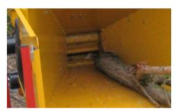
TWIN HORIZONTAL FEED ROLLERS. Two horizontal feed rollers improve performance by grabbing and feeding material to the disc and help in crushing side branches.
