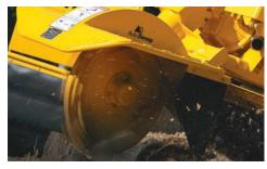
**AUTOSWEEP.** The patented AutoSweep<sup>®</sup> system monitors engine speed and automatically adjusts cutterwheel sweep rate to maximize power to the cutter wheel while reducing engine stress.
