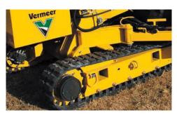
**ZERO TURNING RADIUS.** The planetary traction drive helps provide increased traction while the counter rotating tracks provide tight maneuvering in difficult jobsite conditions.
