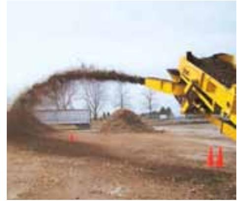
*The HG6000TX blower system is designed for use in clean wood applications. This optional blower features 140-degree rotation and tilt adjustment via remote control to distribute processed material over a large area or into the rear of a chip-hauling trailer. The blower features a heavy-duty impeller assembly with replaceable wear plates and convenient service access.*
