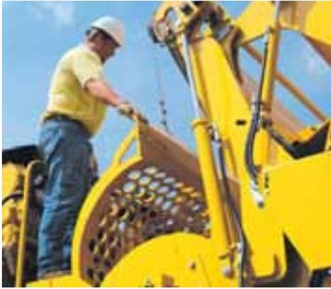
*Easy-access screens are engineered with a top-loading design to allow operators to change screens more easily, and in less time, than conventional screens. A fully hydraulic, moving hammermill / screen cover is easily positioned over the feed table to allow maximum workspace when servicing the mill or changing screens.*
