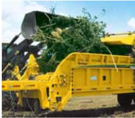
*The patented SmartGrind system and hydraulic feed roller down pressure keep material moving so that loading speed and productivity are maximized. Open-ended, wide feed tables are designed to make over-the-side loading easy and efficient.*
