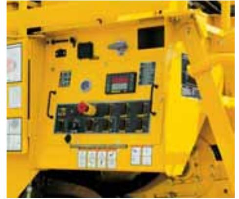
*The standard microprocessor-controlled HPTO clutch is designed to control the starting sequence with the push of a button — no need to bump a clutch. Minimal operator interface is required to initiate the grinding process.*
