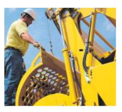
Easy access screens are engineered with a top-loading design to allow operators to change screens more easily and in less time than conventional screens. A fully hydraulic, moving hammermill/screen cover is easily positioned over the feed table to allow maximum workspace when servicing the mill or changing screens.
