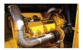
ENGINE POWER. A CAT C32 Tier 2 engine provides 1125 hp (838 kW) of power to meet your jobsite demands.
