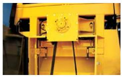
**RELIABLE COMPONENTS.** The poly-synchronous belt drum drive has proven to be a reliable system requiring little maintenance and offering adjustable shafts.
