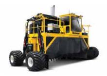
**EASE OF MAINTENANCE.** All grease points are accessible from ground level. Hinged, lockable doors on both sides of the engine provide spacious access for maintenance.
