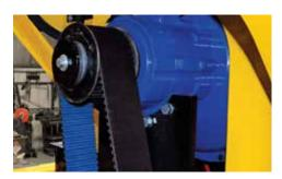
**EXTENDED CLUTCH LIFE.** Engine power is transferred through the hydraulically actuated PT Tech clutch. To help extend clutch life, control software prevents the operator from engaging or disengaging the drum drive at full engine rpm.
