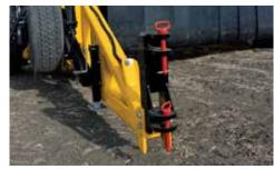
**CONVENIENT TOWING.** An optional low-speed transport kit makes converting between work and transport modes quicker and easier using tow-tractor hydraulics and simple hand tools.
