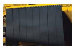
**CONTAINMENT CURTAINS.** Rubber containment curtains draped over the front and back help keep material in the windrow, reducing the quantity and distance of thrown objects.
