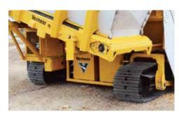
**DUAL TRACK.** Experience more control with the two-speed planetary track drive system - high for transport and normal operation, or low for wet, heavy material.
