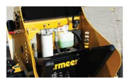
SERVICE MADE EASY. Pop open a panel for access to the hydraulic filter, radiator fill and electrical control board.
