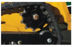
LOWER YOUR COST OF OPERATION with a high mounted track sprocket. The higher mounting reduces premature wear and tear in rocky soil conditions, while the ADI cast sprocket is heat-treated for longer life.
