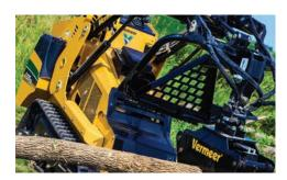
A DUAL HYDRAULIC AUXILIARY option adds a second dedicated low-flow hydraulic circuit to optimize operator efficiency when powering attachments.
