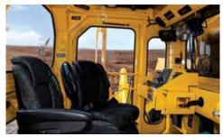
**ELEVATING ENCLOSED CAB.** The cab features dual air ride suspension seats, dual self-contained heating and cooling systems and sound attenuating foam. It is also a rollover protective module (ROPM) and falling object protective structure (FOPS).
