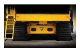
MOBILITY AND STABILITY. The T1655III dual tracks and low center of gravity allow for easy maneuverability and stability over the changing and diverse surface conditions.
