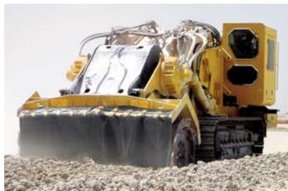
**The innovative Terrain Leveler Surface Excavation Machine** offers unmatched production in a variety of applications, including surface mining, site preparation, over-burden removal, road construction/reconstruction, and soil remediation. The T1255 Terrain Leveler SEM can cut an area up to 12 feet (3.7 m) wide and up to 32 inches (81.2 cm) deep in a single pass.
