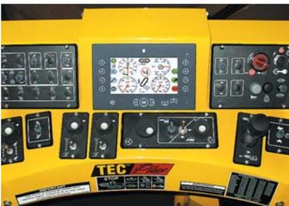
**The new TEC® Plus electronic control system** features CAN bus technology, which utilizes multiple control modules located throughout the machine for real time performance data and advanced troubleshooting capabilities.
