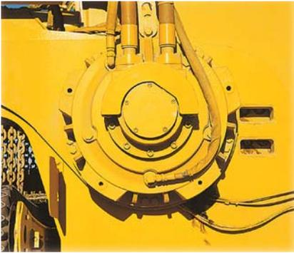
**Dual Rotary Power headshaft motors and a splined headshaft** produce lower speed and higher torque, giving you superior rock penetration and low chain wear for better production results.
