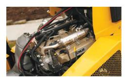
POWER AT THE STUMP. A 40 hp (29.8 kW) T4 Final diesel engine provides substantial power and uses a DOC after-treatment system, which offers reduced maintenance and could lower operating costs.
