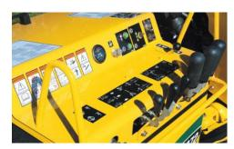
**OPERATOR PRESENCE SYSTEM.** The SC372 is equipped with three operator-sensing control levers that monitor the operator's touch and maintain cutter wheel engagement. When the operator's hands leave the control levers, an automatic disengage and braking sequence will stop the cutter wheel in less than nine seconds. With this safety system, the cutter wheel will automatically stop when the operator releases the hydraulic cutter wheel controls.
