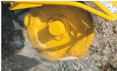
DRIVE SYSTEM. The SC372 features a belt-driven gearbox drive system which provides an efficient transfer of horsepower from the engine to the cutter wheel.
