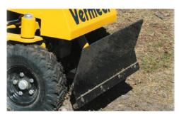
OPTIONAL CHIP BLADE. The blade which is hydraulically controlled from the operator's station, helps eliminate the need for manual chip raking during jobsite cleanup.
