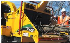
**OPERATOR SAFETY.** Combined with the patented Bottom Feed Stop Bar is a four-position upperfeed control bar with dual stop positions and forward/reverse feed positions. Mounted over the feed table, this enables the operator to stop the feed rollers and select forward or reverse operations. Dual reset/hold-to-run buttons allow the operator to readily reset both bars.
