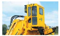
**ELEVATING ROPM CAB.** The spacious elevating rollover protective module cab features LEXAN® glass, filtered and pressurized air, heating and air-conditioning. The cab's vantage point allows a virtually unrestricted view of the boom, trench and conveyor.
