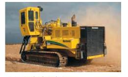
**ELEVATING ROPM CAB.** The elevating rollover protective module cab features LEXAN® glass, filtered and pressurized air, heating and air-conditioning. The cab's vantage point allows a virtually unrestricted view of the boom, trench and conveyor.
