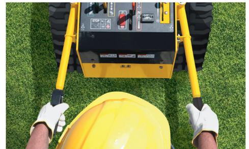
**VZ STEERING.** Instead of additional levers and steerable wheels, the operator can turn the machine using only the handlebars. These bars also provide additional leverage when operating in difficult terrain.
