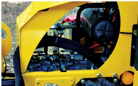
**OPERATORS, START YOUR ENGINE.** The 25 hp (18.6 Kw) Kohler electronic fuel-injected (EFI) gasoline engine offers improved fuel economy reducing greenhouse gas by an average of 25% - as compared to conventional carbureted engines. And, best of all, makes choke cables obsolete. Simply put, it's time to start your trencher like you would your car.
