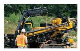
KNUCKLEBOOM CRANE. Optional knuckleboom crane mounted on either side of the base anchor easily maneuvers heavy tooling, reducing need for support equipment.
