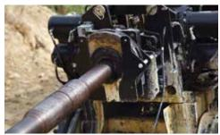
VISE. The sliding vise moves 35.4" (89.9 cm) to help operators position the vise for maximum efficiency when reaming or pulling product.
