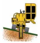
**OPTIONAL AUTO TILT TRACK.** An oscillating track frame allows the track to follow the ground's contour ensuring a vertical trench on slopes up to 10 degrees.
