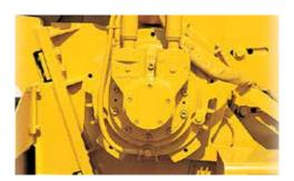
ROTARY POWER TRENCHER DRIVE MOTOR. A rotary power trencher drive motor and splined
