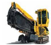
**ELEVATING ROPM CAB.** The elevating rollover protective module cab features LEXAN® glass, filtered and pressurized air, heating and airconditioning. The cab's vantage point allows a virtually unrestricted view of the boom, trench and conveyor.
