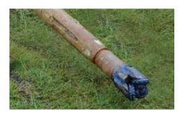
**DRILL BIT OF CHOICE.** Designed to optimize operation in a variety of conditions, choose from a wide range of drill bits and a specially designed dual rod drill head offered in three different bent sub arrangements.
