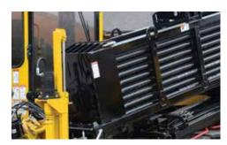
ROD CARRYING CAPACITY. The D36x50dr Series II carries up to 500' (152.4 m) of drill rod, reducing the need to load additional rod when performing extended bores.
